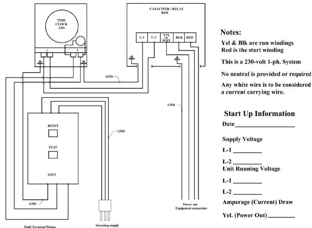
Field Terminal Wiring Wiring Screws Shall be tightened to 20 in/lbs of torque Use Copper Conductors Only
