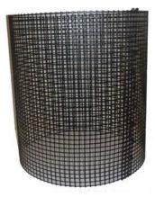
Step 3 Attach the mesh cylinder to the inside circumference of the hole in the center of the float. There are 1/4-20 brass inserts molded into the float to attach the debris screen. Secure the debris screen with stainless steel  $1/4-20 \times 1/2$  inch hex head screw and a 1/4 inch stainless steel washer.
