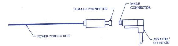
Connect the power cable to the unit. A packet of dielectric grease has been provided. Apply the dielectric grease into the water tight connectors to aid in the installation of the connectors and to provide additional moisture resistance. Insert the female connector of the power cord into the male connector on the unit and tighten the jam nut hand tight. (Do not over tighten as damage can occur)
