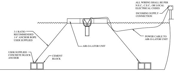
Position the float where desired and drop one anchor block and then the other at an angle to the float. (See the diagram below)
