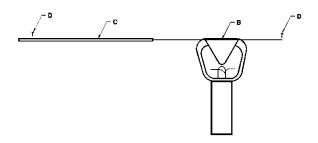
STEP 3) Separate the two 10-foot sling ropes setting one of them aside. Insert the remaining sling rope. Select the rope end opposite the stainless steel washer and rubber bushing into the diffuser support tube hole inside the "funnel shaped" area. Do the same with the remaining sling rope and pull through the diffuser until the rubber bushing is in the diffuser support hole and the stainless washer is against the inside of the funnel shaped diffuser.
