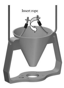
STEP 4) If the flotation is to be used during ice melting you must insert the loose sling rope ends into the flotation from the bottom of the float up and through the molded holes opposite the mooring ropes points.
