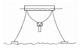
STEP 5) At this point the selection of the operating depth is to be accomplished. Generally the depth of the propeller is the preferred point of reference since the propeller is what does the work and is commonly set at 5-foot of water depth. It may be desirable to select a different depth, however positioning the propeller any deeper than 8-feet of depth is not recommended. The motor at no time is to be operated while in mud, rocks or sand. Damage may result to the motor and propeller.
