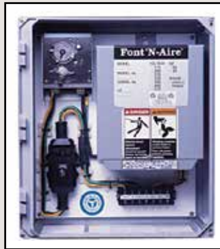
ETL CONTROL PANEL ANSI/UL508 control panel with time clock equipment leakage circuit interrupter (ELCI) and motor controls placed in a NEMA 4X enclosure
